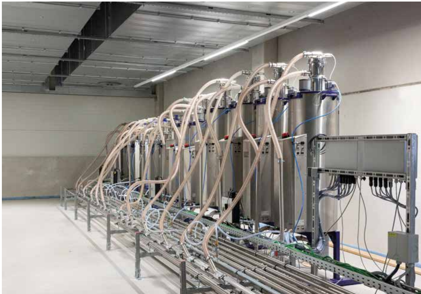
Drying plant for plastic material, with vacuum valves
